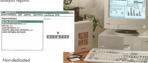
Conventional charging systems require the PC to be dedicated to this application. The Alcatel 4715 AX does away with this constraint. The processing module is equipped with its own processor, its own memory (RAM) and a backup battery. Your PC thus retains all its characteristics for your standard applications, without any disturbance. You can switch your PC on or off normally.
